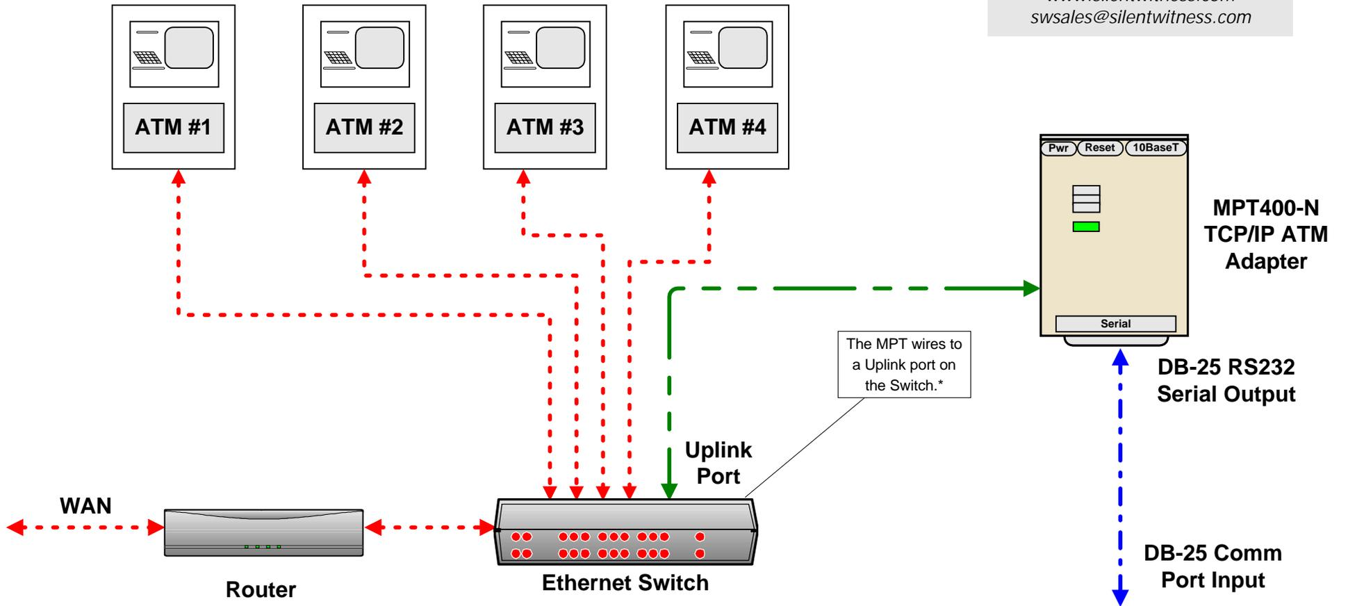
The MPT wires to a Uplink port on the Switch.\*
