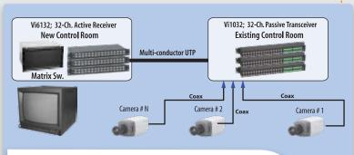
Use passive hubs in the existing control room and active hubs in the new location. Video can be sent over 3,000 feet (915m) with video equalization and ground loop isolation in the new location. This saves installing huge bundles of coax and expensive line drivers. All video signals travel across a small multipair cable.
